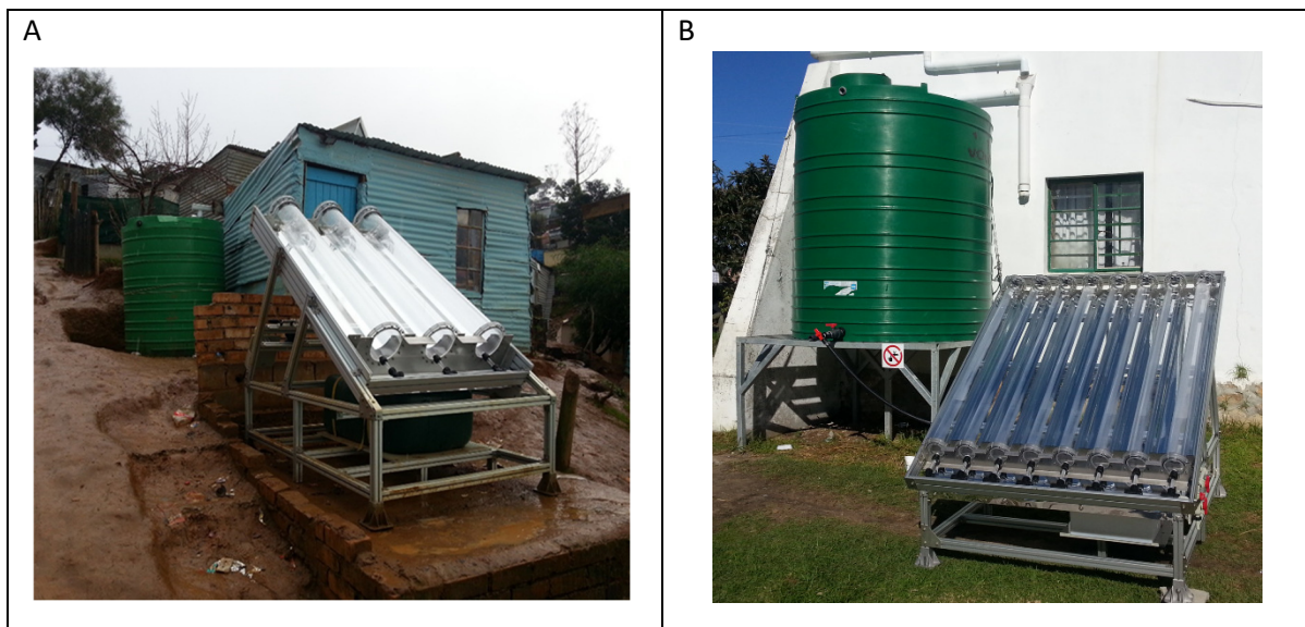
Figure S1. Prototype I (A) and Prototype II (B) of the polymethyl methacrylate (PMMA) tubular solar reactors at Stellenbosch, South Africa.
